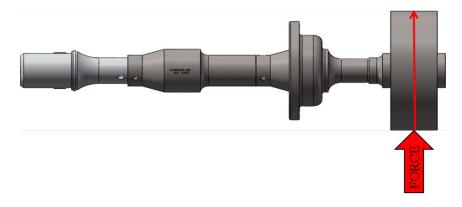
One of the key advantages of the rotary sonotrode is the ability to achieve very high amplitudes and operate in contact with other surfaces. Impact force to the radial surface of the rotary horn does not damage the converter.
